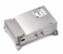
4-input (III+DAB, IV, V, UHF) multiband TV indoor amplifier with 43dB gain and up to 125dBµV output level on UHF band, separate amplification with independent level adjustment (20dB) for each input and low noise figure. T2 technology with UHF cut band for LTE 4G @790MHz and 5G @694MHz.
